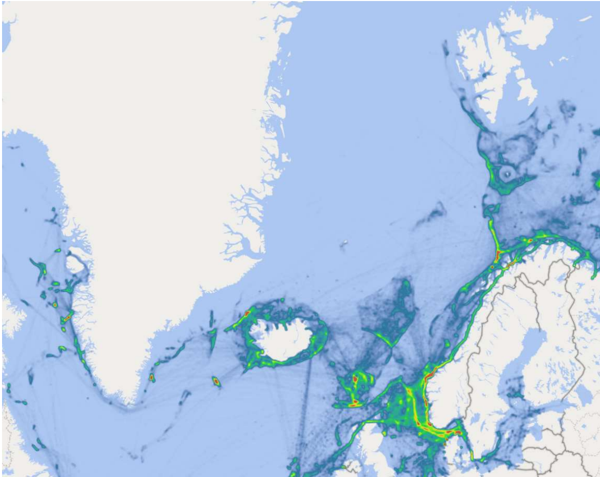
Figure 3-11. Traffic patterns for all fishing vessels – 2019. Colouring indicates fuel consumption density at the given geographical location.
