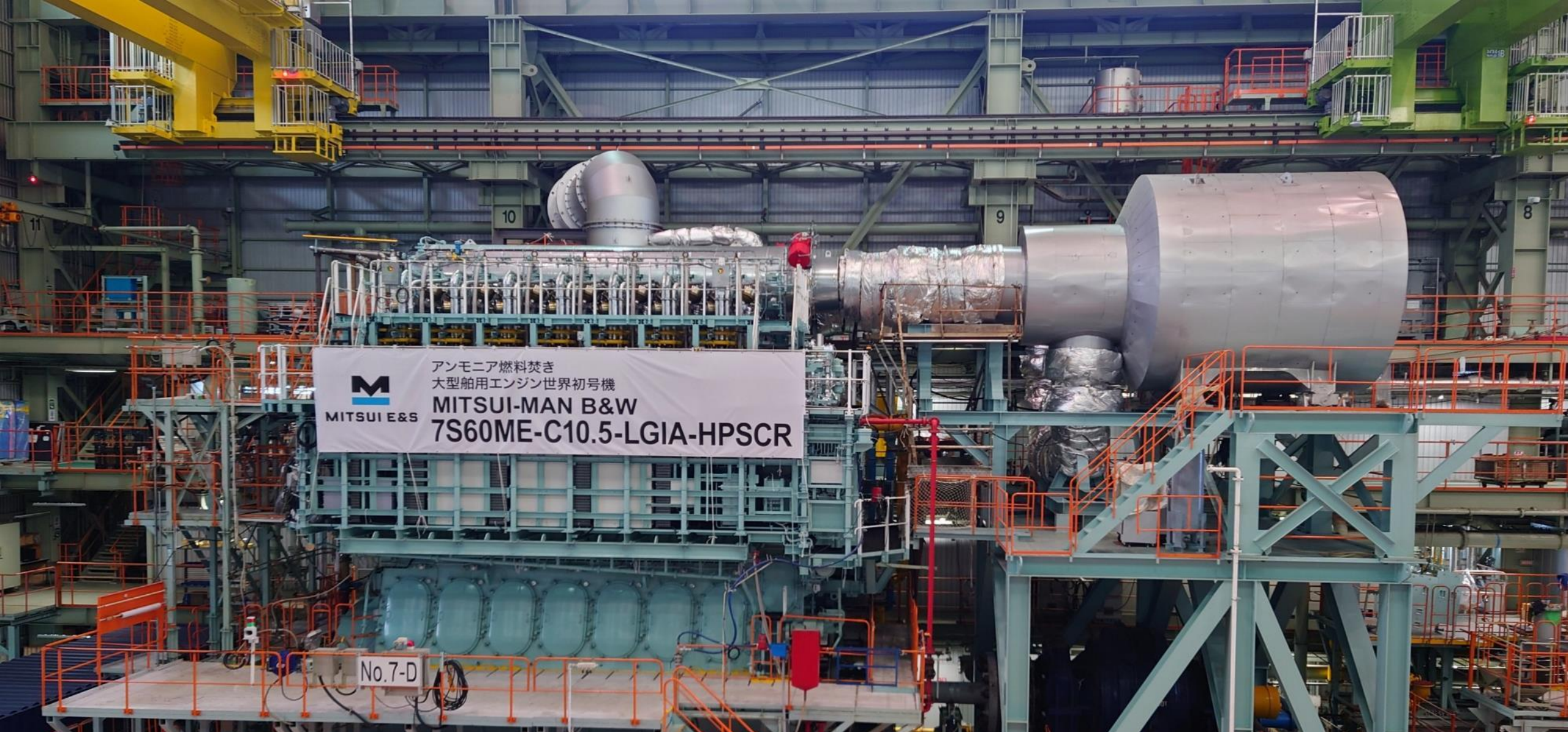
7S60ME-C10.5-LGIA at MES has been operated on Diesel. Currently the ammonia auxiliary systems are being finalized. Delivery time schedule will be pending shipyard delivery schedule.
