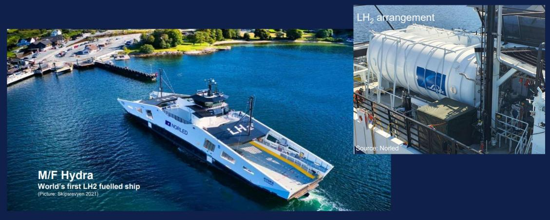
In operation on batteries only, 2021. Sailing with hydrogen fuel cells since March 2023.
