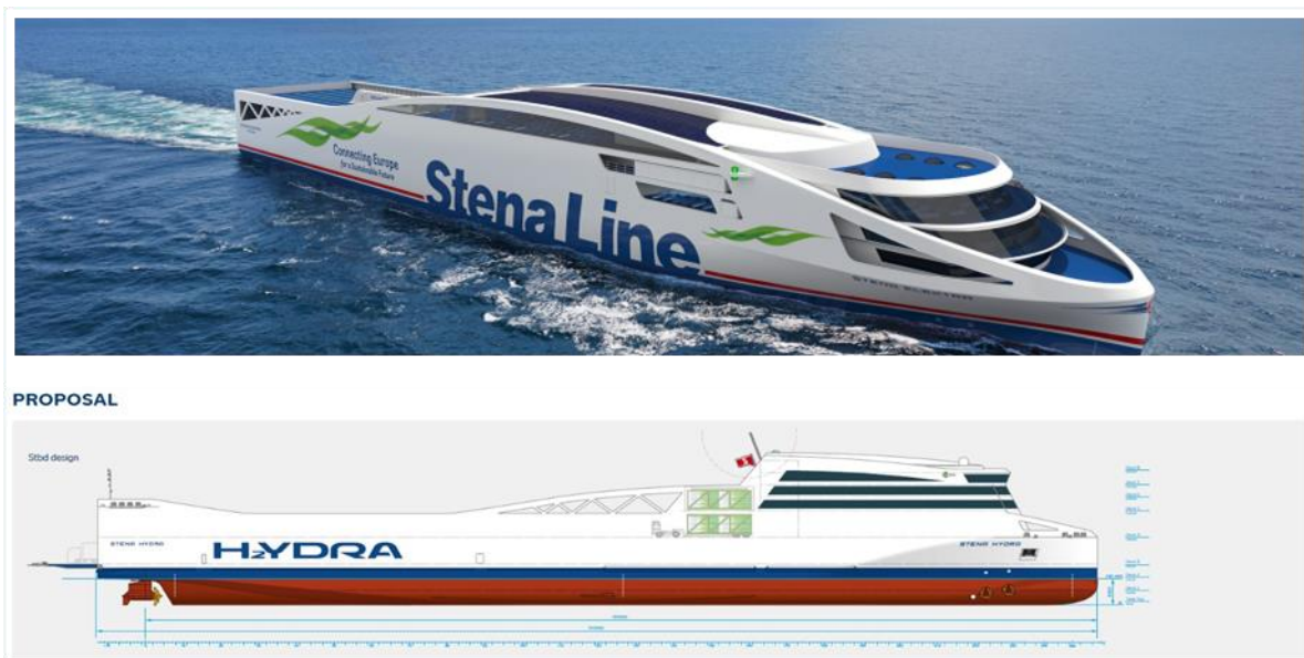
Figure 2. Illustrations from earlier concept studies by Stena and other parties. Stena Electra (battery electric) and Stena Hydra (hydrogen – fuel cell). Illustrations from Stena.
